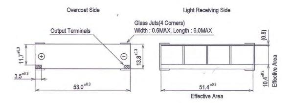
Note: Glass Substrate Thickness : 1.1mm
